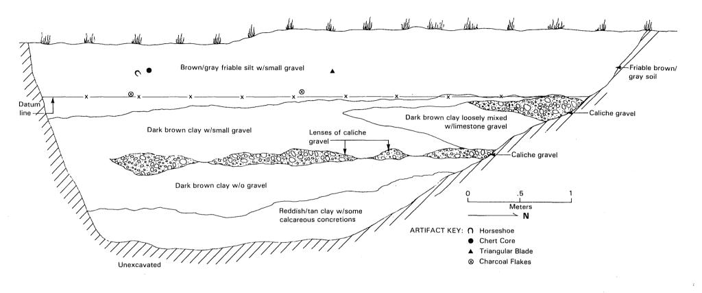
Figure 2. Profile of Backhoe Test Unit 14.
