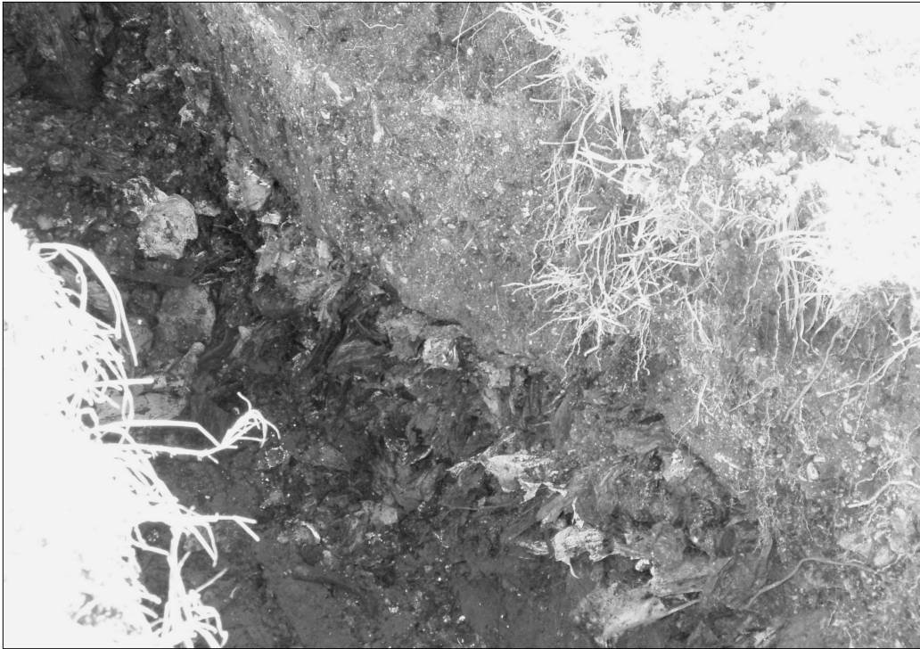
Figure 4-4. Landfill material encountered in Backhoe Trench 2.
