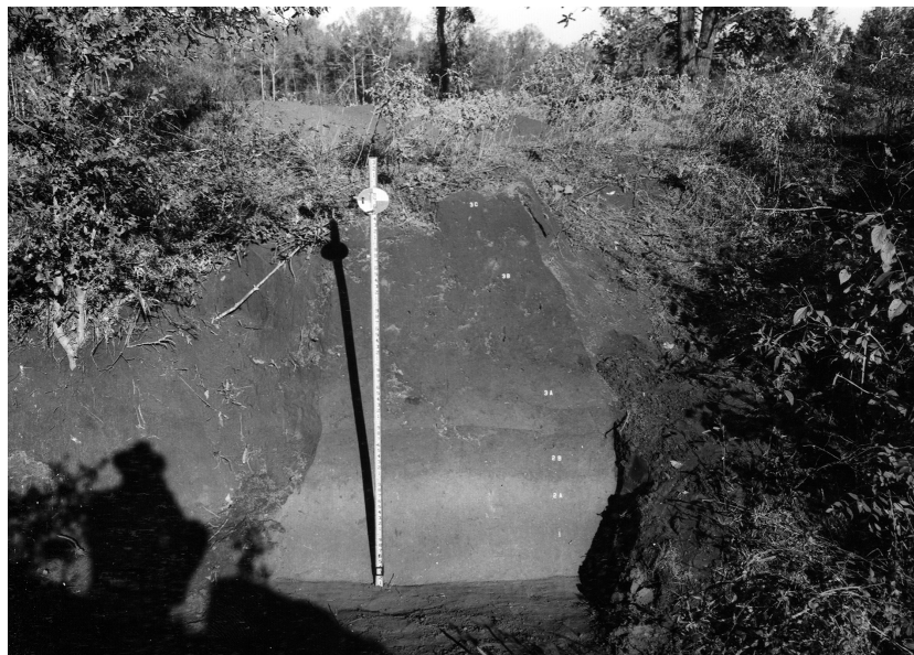
Figure 36: Sawmill Site, profile showing soil zones. Note buried humus zone, labelled 2B.
