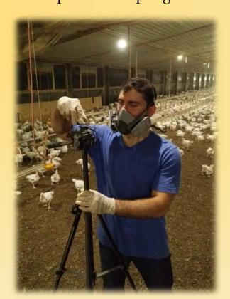
Setting up a Colorimetric NH<sub>3</sub> Sampler Tube Inside One of the Chicken Houses for Aerial Exposure Sampling
