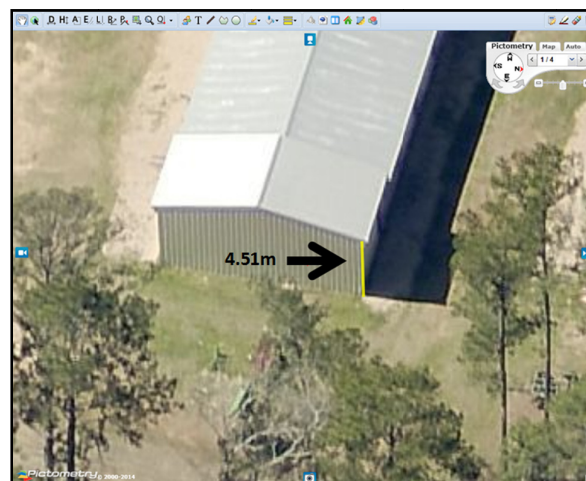
Figure 3. Example of estimating building feature height within the Pictometry web-based interface.
