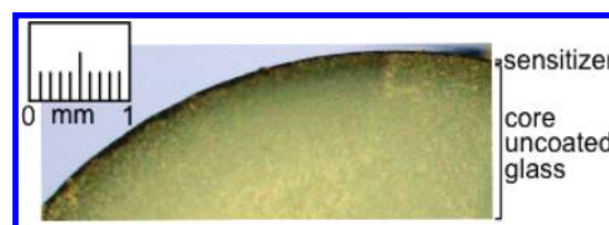
Figure 3. A low-magnification (10×) cross-sectional optical image. The dark green thin coating shows the depth of 1 accessed into PVG. The image shows ~0.08 mm penetration depth on the outer face of the cylinder-shaped PVG cap 1 (diameter 5.0 mm × length 8.0 mm).
