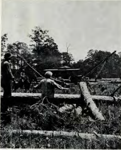
Figure 6. From temporary spur rail-road tracks, tongs on long cables were dragged into the woods by horses, to be pulled back by powerful engines, with loads of logs. Thompson and Tucker Lumber Co.
