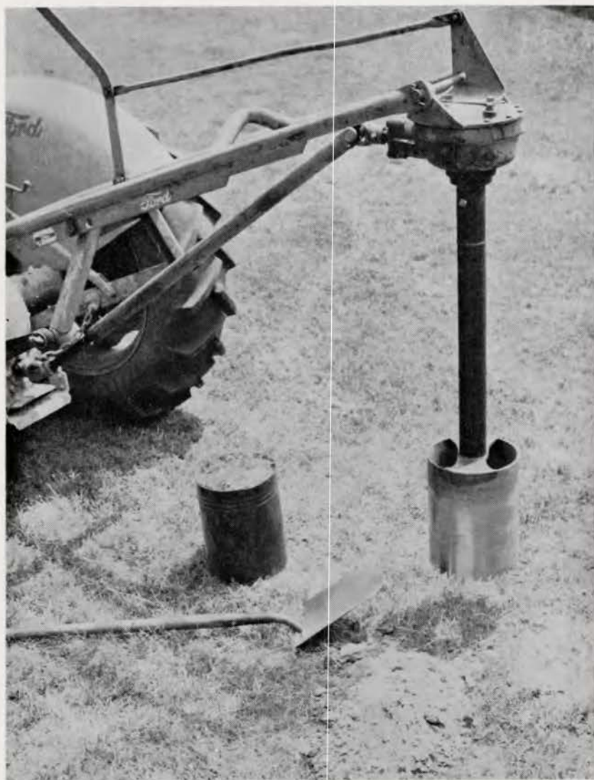
Figure 3. Power cutter for large undisturbed soil cores.
