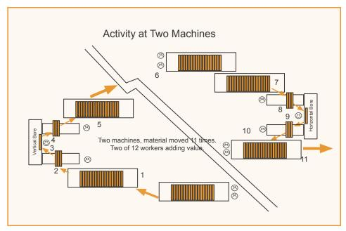
Figure 2. The original batch-processing layout at the vertical and horizontal boring machines. Smiling faces indicate workers who add value while frowning faces indicate workers who are not engaging in a value-added activity.
