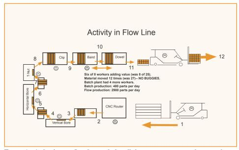
Figure 4. Airline's new flow-line includes all the operations required to complete the product-group parts.
