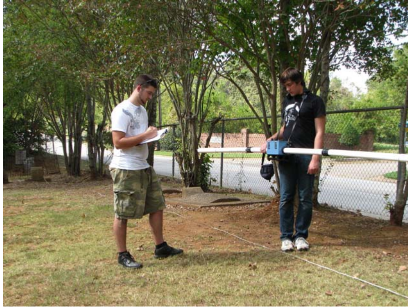
Figure 3: Matthew Worrell (left) recording data points from the EM-31 held by Zachary Overfield (right).
