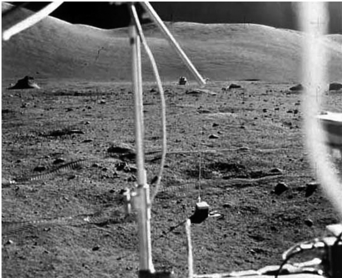
Figure 4. One of 8 explosive packages (black box with a white lid and aerial in the foreground) deployed in the Taurus-Littrow valley as part of the Apollo 17 active seismic profiling experiment. This view is from the LRV towards the Sculptured Hills (see Fig. 3). The lunar module, where the seismic array was set up, is visible in the distance (NASA).
