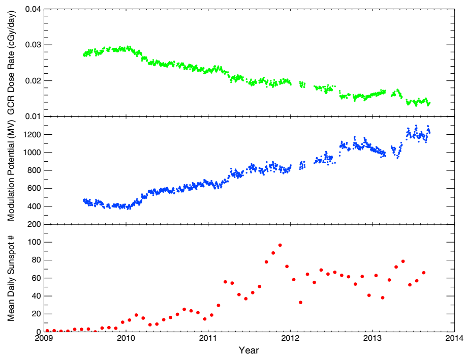
Figure 2. Plot of GCR dose rate and modulation potential at the Moon during the LRO mission as the Sun transitions from minimum to maximum. Sunspot number as provided by the Solar Influences Data Analysis Center (SIDC) is shown to provide context within the solar cycle. Plot has been updated from the one shown by Joyce et al. [2013].
