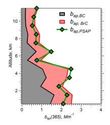
**Figure 2.** Vertical profiles of estimated black carbon (BC) and BrC absorption coefficients, along with the inferred ambient aerosol observed total absorption (PSAP), all at 365 nm. Uncertainty associate with each parameter was 45% for  $b_{ap,BrC}(365)$ , 22% for  $b_{ap,BC}(365)$ , and 29% for  $b_{ap,PSAP}(365)$  (details in supporting information).
