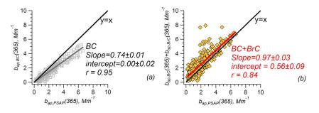
Figure 3. Closure analysis of absorption coefficients at 365 nm between (a) BC and (b) the sum of BC and BrC, each compared to total aerosol absorption from PSAP data. Orthogonal distance regression fit results are shown.
