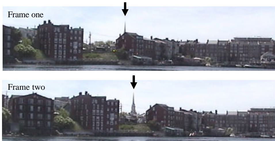
Figure 4: Two video frames taken from roughly 20 meters apart. These frames illustrate a geometric problem of parallax: there is no one location that a given image with prominent features at different depths can be properly placed in a scene. The church steeple appears in one place with respect to the other buildings on the coastline from one vantage point, but in another place from another vantage point not far away.
