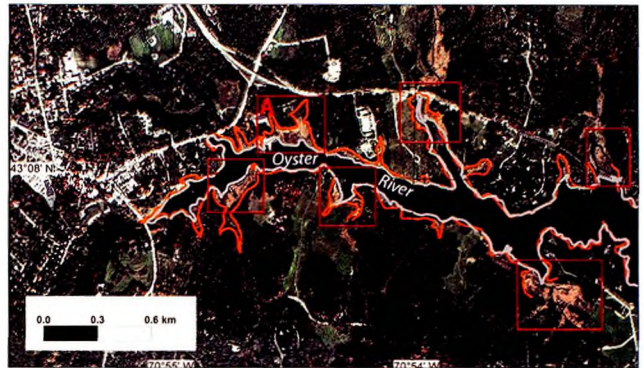
Figure 12: Differences in Mean High Water coastlines from 1913 (orange) and 1953-54 (grey) surveys. The red boxes indicates areas where it is clearly visible that the 1953-54 coastline is located more seaward. A photograph taken of the area in the box marked A is shown in Figure 13.
