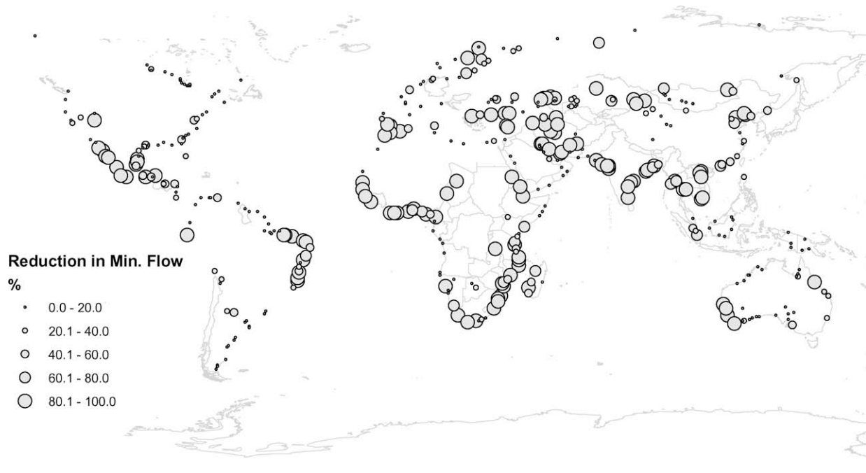
Fig. 8. Modelled reduction in minimum monthly river discharge at outlet caused by operation of SR's to supply irrigation water to croplands for the period 1998–2002 for 416 river basins ( A > 25,000 \text{ km}^2 ) with cropland area.
