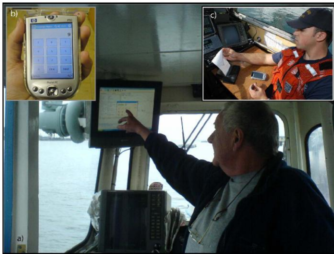
Figure 5. Simplified task-specific user interfaces can make using AIS much easier. a) The Thames River in England requires ferries to notify the local Vessel Traffic Service (VTS) with the number of passengers via AIS. b) With the right interface, an AIS application can be ported from fixed computer to a handheld. c) USCG Los Angeles station personnel using a PDA while working on a smaller patrol boat. Integrating AIS into these mobile devices can aid in incident response. Images from [33] and USCG.
