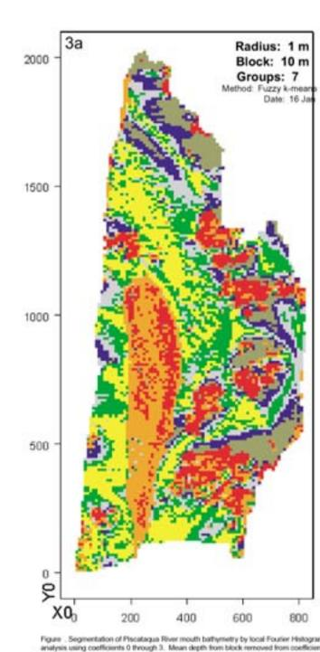
Figure . Segmentation of Piscatagua River mouth bathymetry by local Fourier Histogram (LFH) analysis using coefficients 0 through 3. Mean depth from block removed from coefficient 0, therefore difference from mean depth used to remove mean depth effect from results. LFHs. LFH block size = 10 by 10 meters. distogram bin maximum values set automatically using
