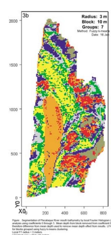
analysis using coefficients 0 through 3. Mean depth from block removed from coefficient 0. therefore difference from mean depth used to remove mean depth effect from results. LFH: LFH block size = 10 by 10 meters. Histogram bin maximum values set automatically using: histrau(i)=meancoef(i)=vercoef(i).
