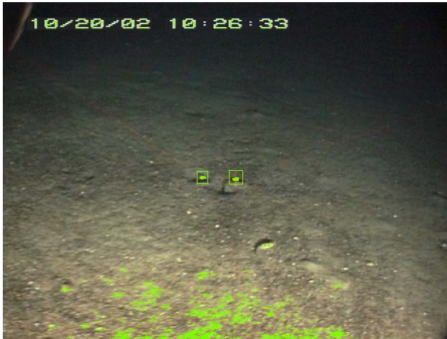
Fig. 1. Results of the classification of an entire frame (notice that the digits at the top of the frame were classified as laser dots too).
