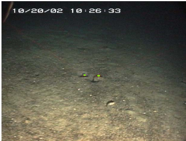
Fig. 3. An example of pixel classification with geometrical constraints applied (greenish pixels were classified as parts of laser dots)
