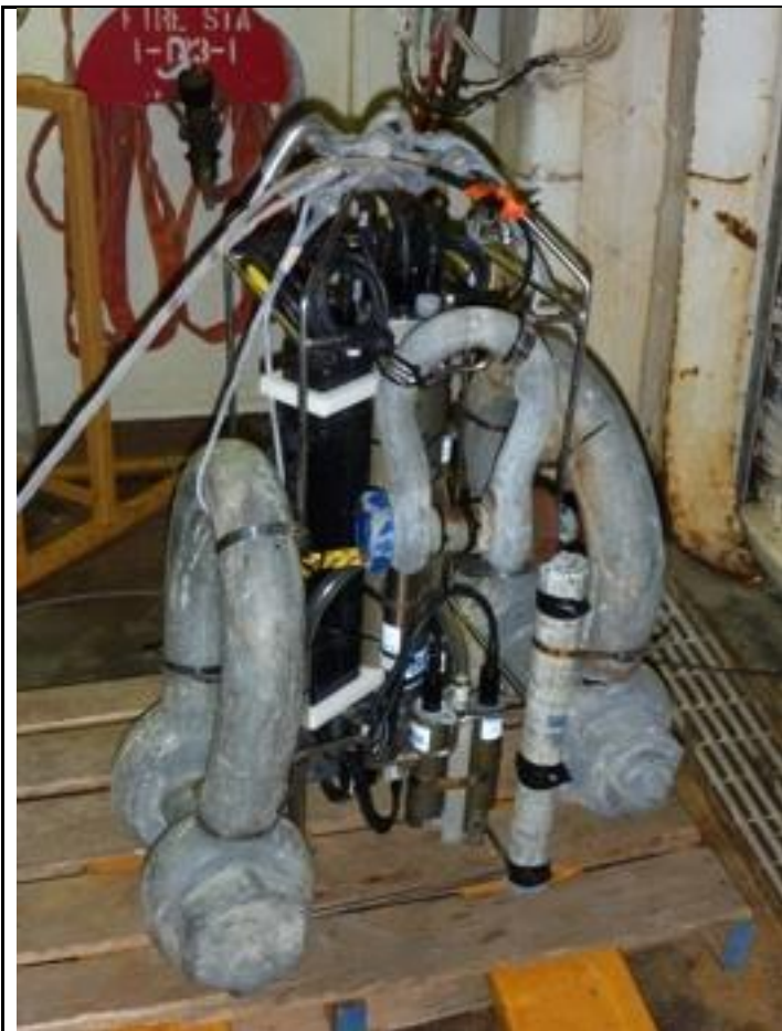
Figure X: Photograph of the large shackles weights added to the CTD package to achieve a reasonable weight.
