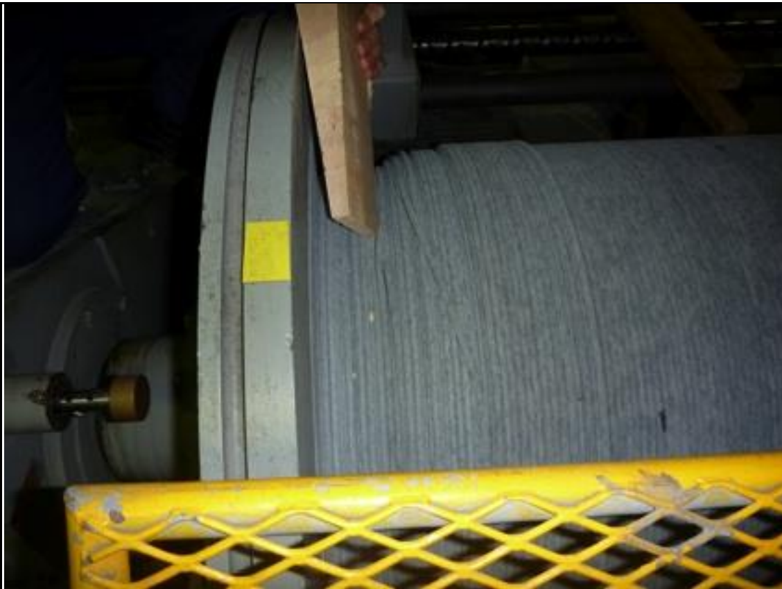
Figure X: Photograph of the cinched wire on the CTD drum.
