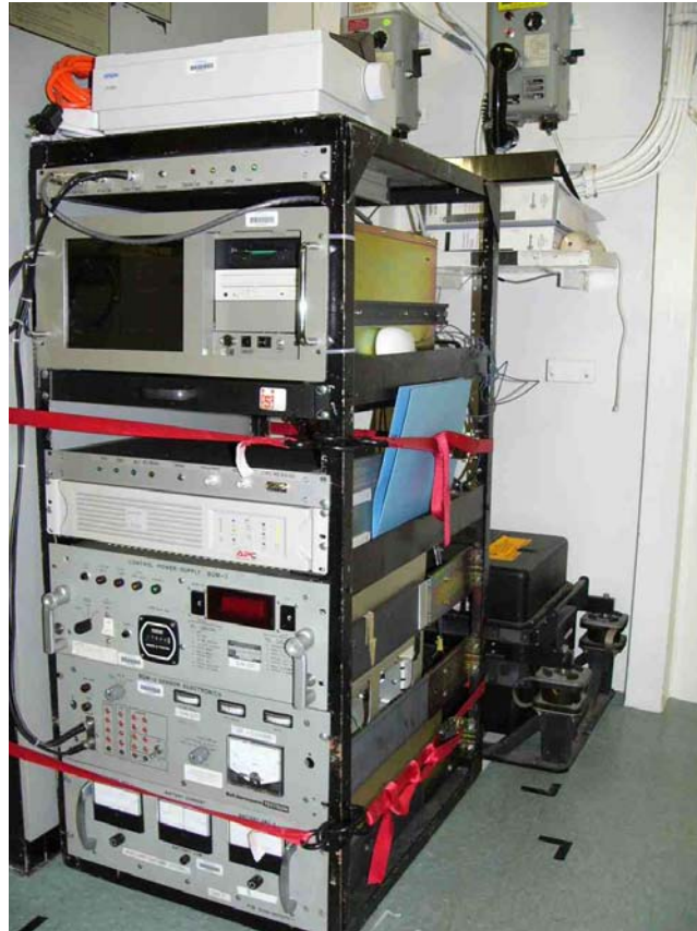
Figure 5 – Gravimeter as installed for Summer 2004 program on USCG Healy.
