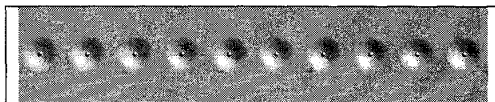
Figure 6a: Sun-illuminated view of the terrain ensnified (1000m long by 200m wide). Source lies to the centre left, elevated 500m above the surface. Each 5m deep, 80m wide depression has a 5m high, 10m wide knoll at its centre.
