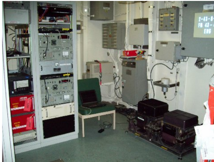
Figure 86. Two Bell BGM-3 gravimeters as installed in February 2008 on USCGC Healy. Electronics for both systems are housed in the vertical rack. The two shock mounted black platforms are on the right, mounted on a metal plate attached to the deck.
