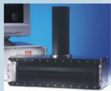
Fig. 1. Sonar head of Reson 8125 multibeam. Transmitter (vertical) is approx. .4m while receive array is approx. .5 m in length.
