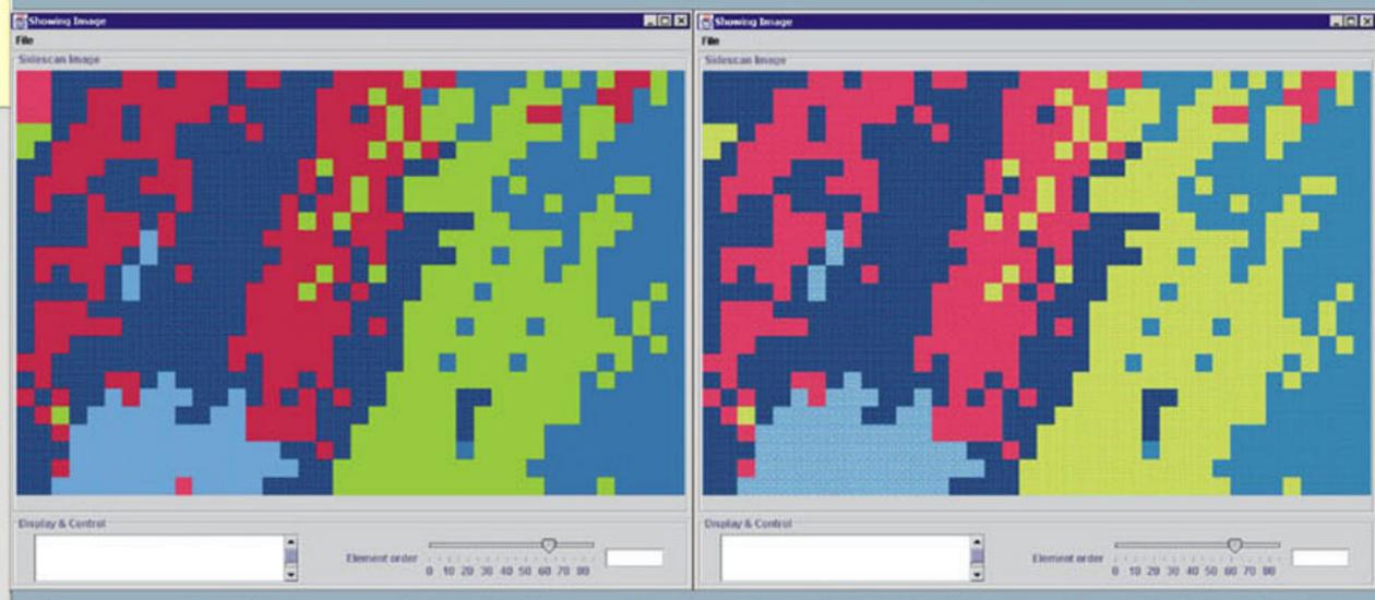
n unsupervised K-means clustering algorithm was implemented using backscatter strength vs. the best-estin igle as the elements in feature space. In this approach, the geometric corresponding cluster- representative was computed as an element of the feature space at each iteration.
