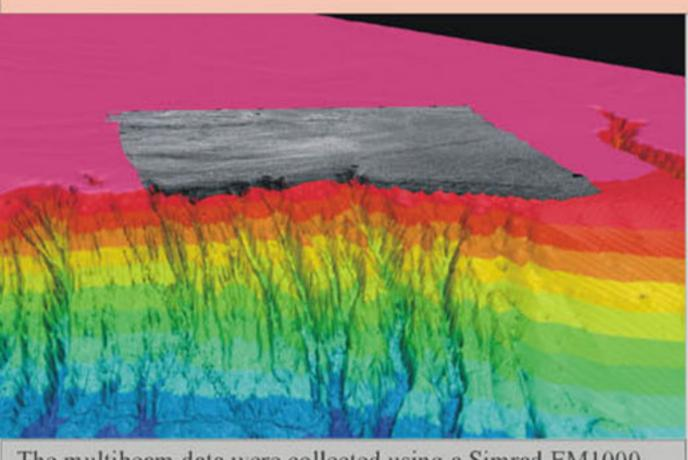
The multibeam data were collected using a Simrad EM1000 system, which provides both bathymetry and backscatter at 95 KHz. A small subset (13 x 20 km) of the NJ multibeam survey was selected as the focus of this research
