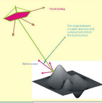
surface normal can be defined by  $[p = \frac{\partial f(x, y)}{\partial x}, q = \frac{\partial f(x, y)}{\partial x}, -1]$  at the point {x, y} on the surface z = f(x, y). The pair (p, q) represents the surface orientation at  $\{x, y\}$ . The bi-quadric fit involves finding the six coefficients of the polynomial
