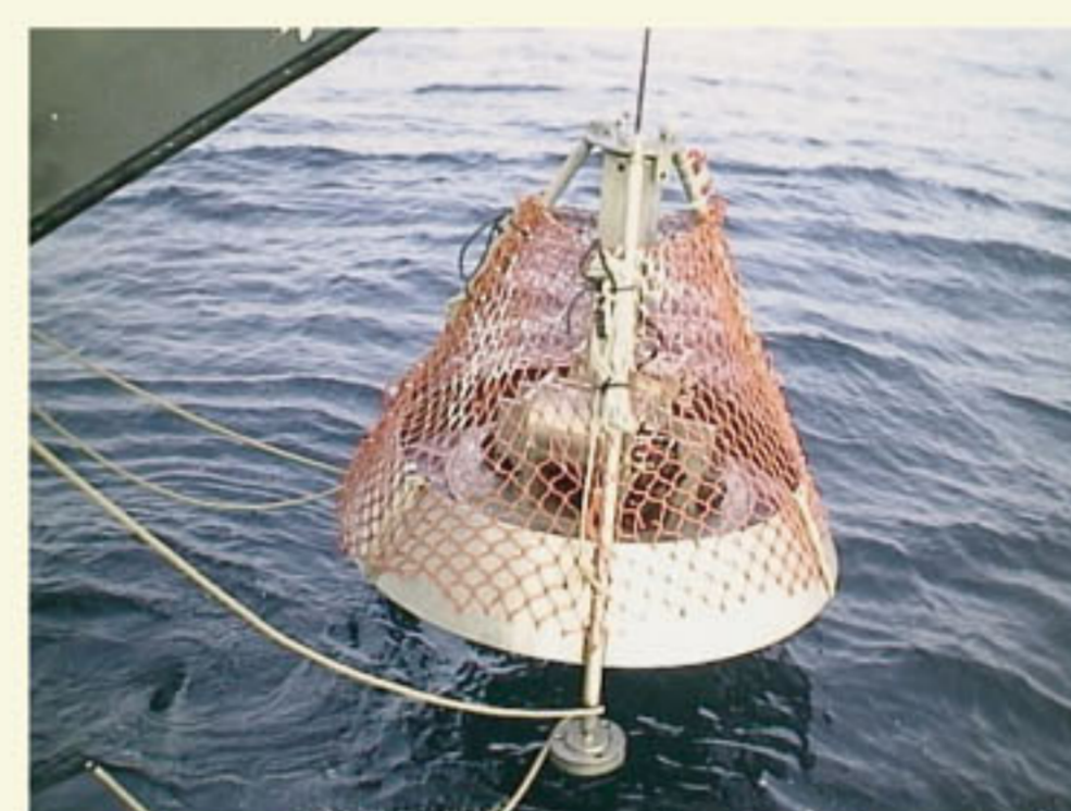
Figure 2. Deployment of ISSAP probe. The ISSAP instrument weighs approximately 275 kg, has a height of 1.5 m, and a 9.4 m square footprint. The outer frame consists of a protective tripod reinforced with a tapered skirt. Articulated tripod feet allowed for vertical probe insertion on slopes up to 20 degrees.
