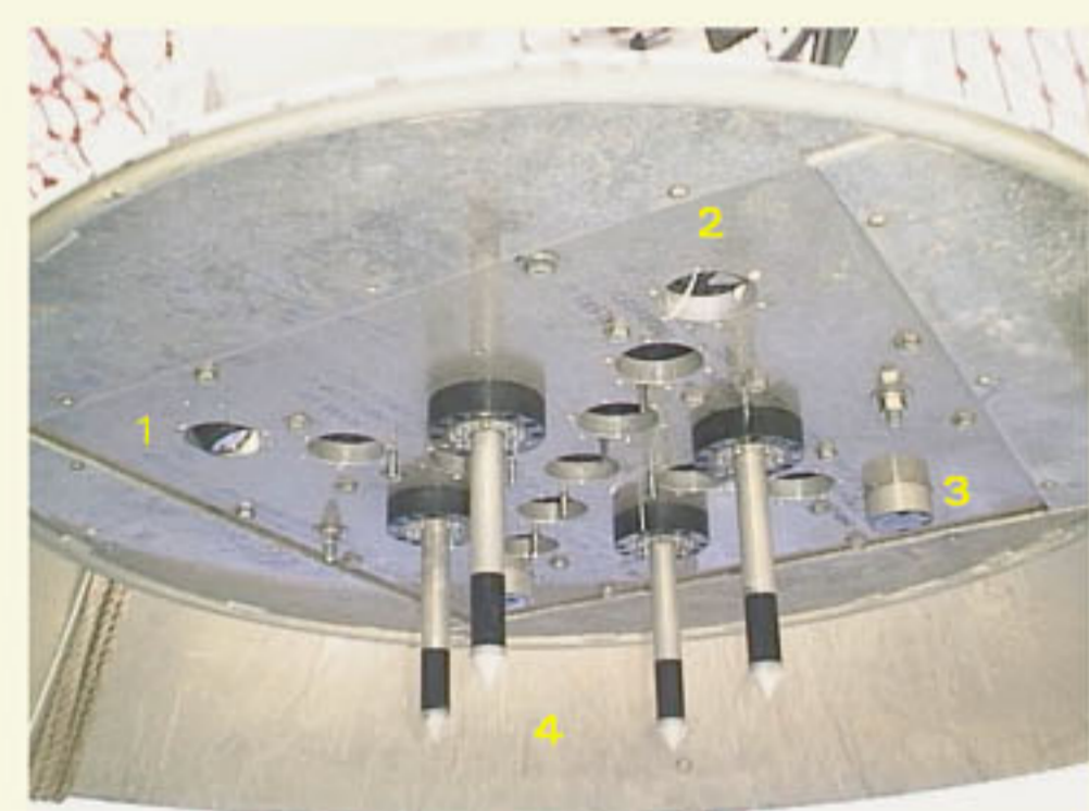
Figure 1. Arrangement of transducer probes on ISSAP and method of mounting. Also shown are the 1.) color video camera, 2.) light, 3.) altimeter transducers and 4.) 65 kHz compressional wave probes (4) with path separations of 20 and 30 cm.
