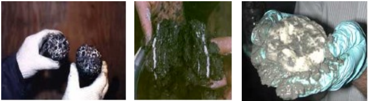
Figure 5.3. Photographs of methane hydrate as nodules, veins, and laminae in sediment. Courtesy of USGS ( http://geology.usgs.gov/connections/mms/joint_projects/methane.htm ).
