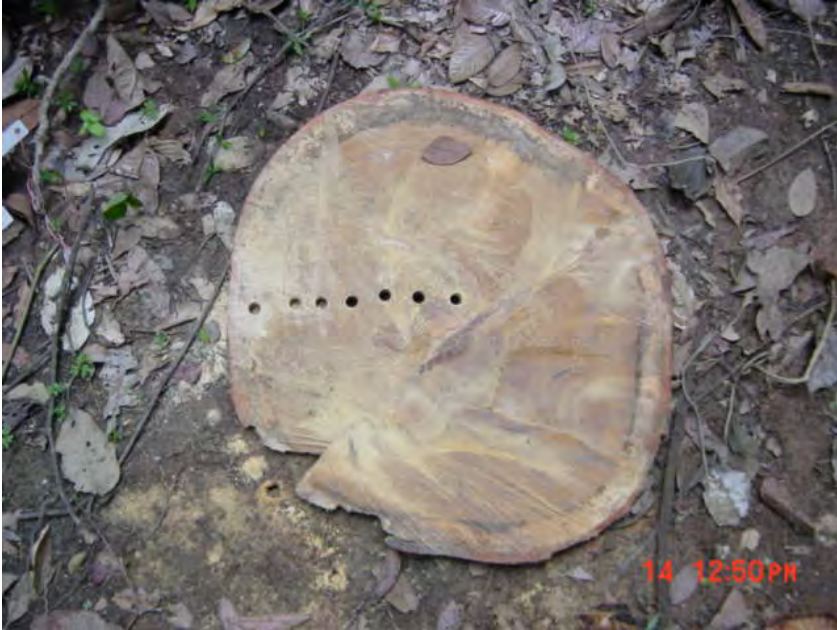
Image 3. Multiple samples extracted from a section of fallen necromass using the tenon extractor.
