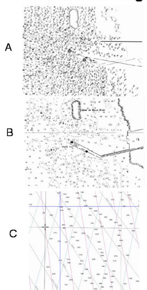
Not every data point is used in the final product. "A" was thinned to create "B". Notice the other chart snippets; "C" scaled for open ocean, and to the far left, scaled for coastal use. Does the pattern, or lack of soundings adequately convey the amount of data to the user?
