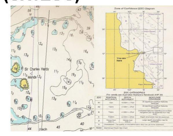
The hydrography in this example is not listed by source, but by an accuracy/completen ess criterion. While a more scientifically correct attribution of the data's uncertainty, is this a useful tool for the Mariner?
