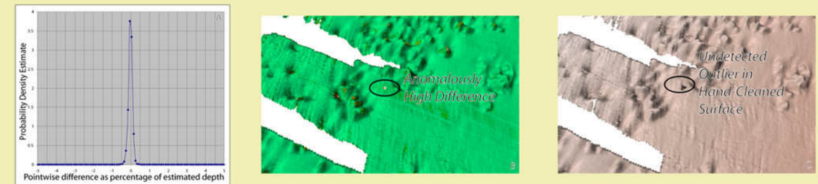
Figure 6: Comparison of surfaces. CUBE's surface estimate closely matches the hand-generated surface (A), and where there are significant differences (B: differences color-coded over CUBE's depth estimate), they typically indicate an outlier remaining in the hand-cleaned dataset (C). The red-white transition is at 2.3% of water depth, approximately the limit for IHO S-44 Order 3 survey (for depths over 200m).
