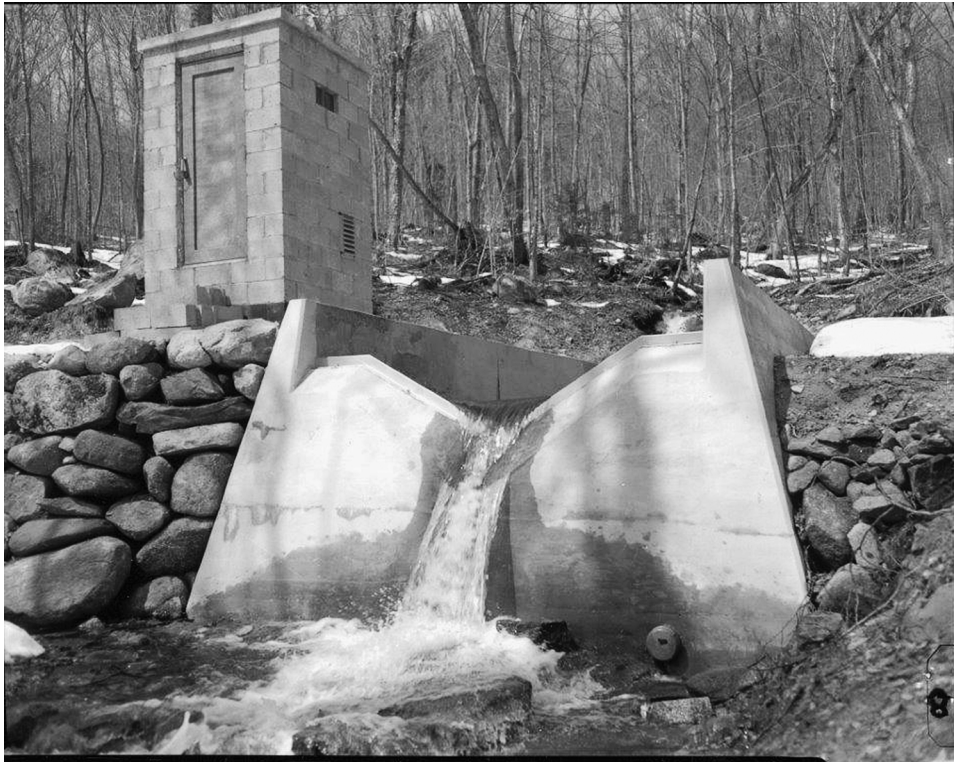
PLATE 1. V-notch weir for measuring stream discharge from a small watershed at the Hubbard Brook Experimental Forest, New Hampshire, USA. Photo credit: Northern Research Station, USDA Forest Service.
