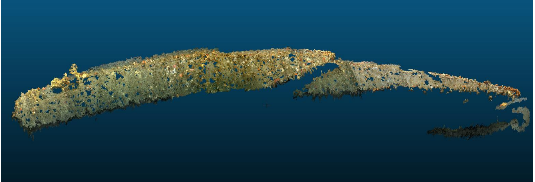
Figure 34. Full point cloud from all the images of top view sequence after bundle adjustment (Perspective 2).
