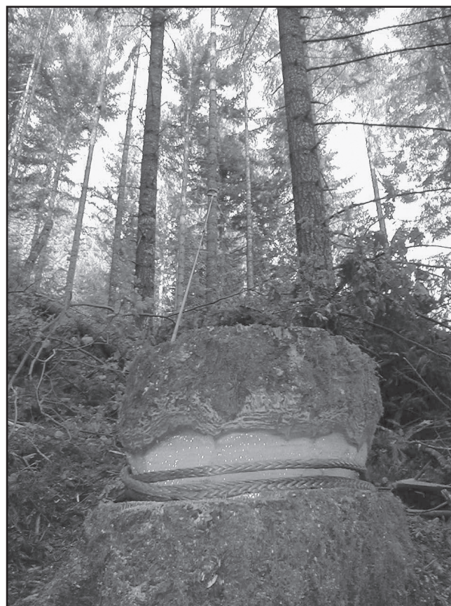
Synthetic rope guyline anchor stump.
