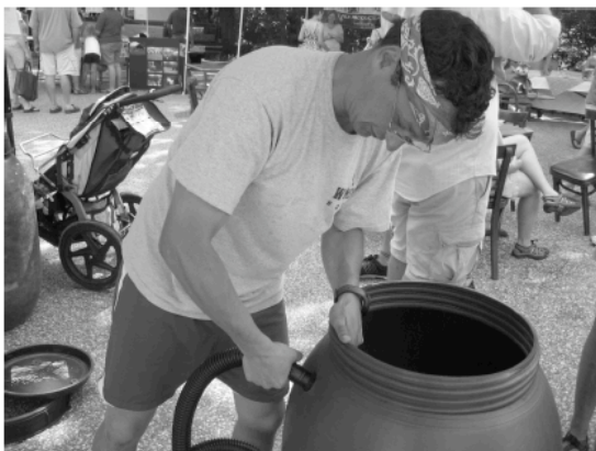
Step 11: Attach discharge hose to adapter
