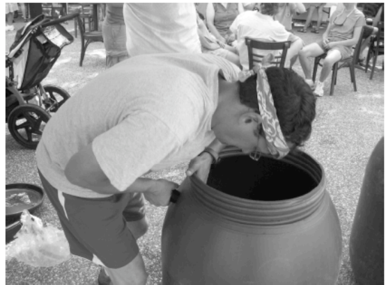
Step 10: Screw 1 1/2" adapter into the hole
