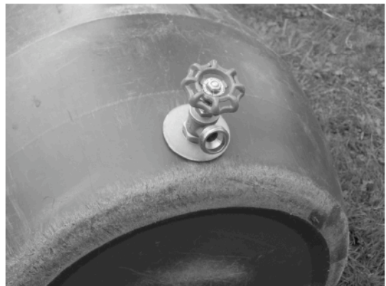
Step 6: Screw spigot into hole
