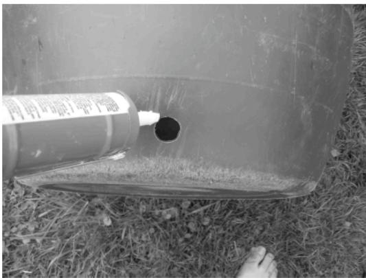
Step 3: Apply a thin bead of caulk around the hole
