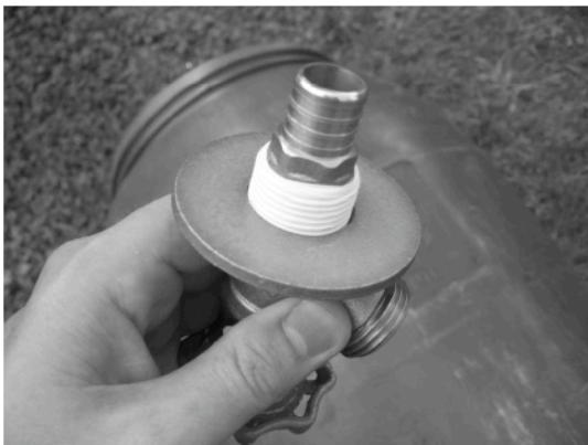
Step 5: Place washer on end of spigot
