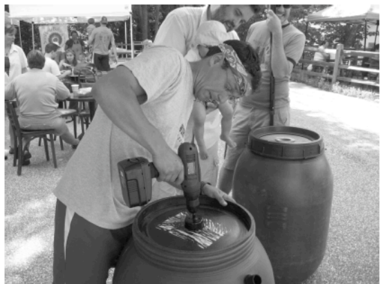
Step 12: Use 2 1/2" hole saw to drill a hole in the top/lid of the barrel
