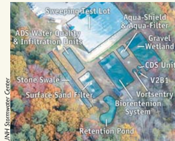
UNH Stormwater Center's Treatment Units
