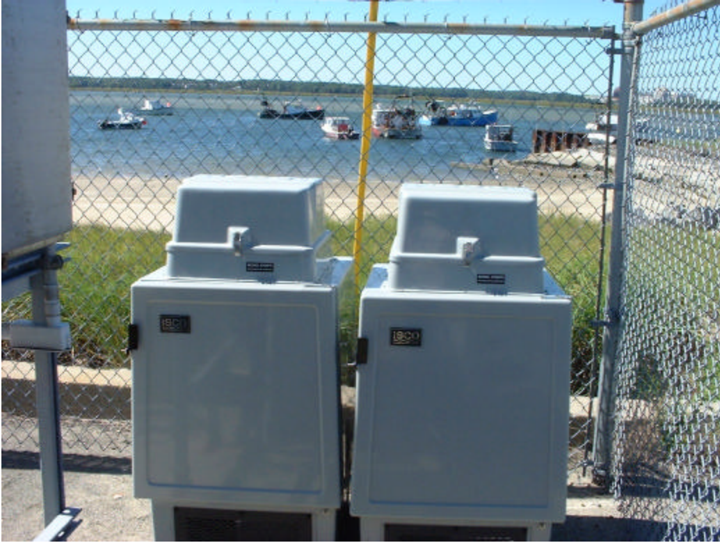
Figure 6 Autosamplers in enclosure at monitoring site.
