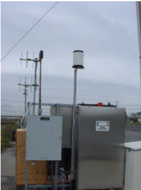
Figure 4 Monitoring site with view of rain gauge.
