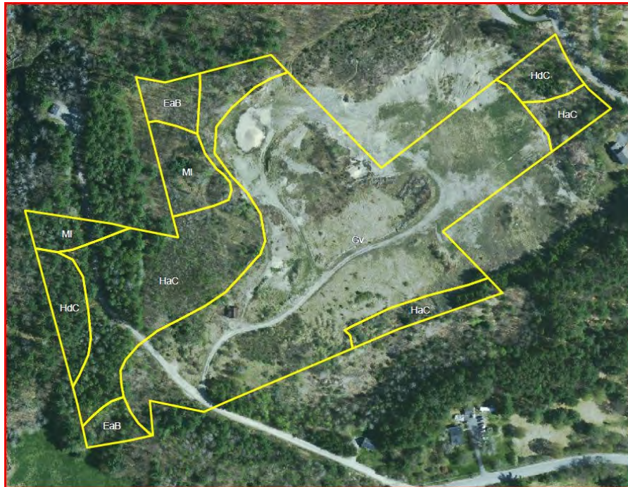
Figure 2 Soils re-drawn from NRCS Strafford County Soil Survey Data (2001) to reflect extent of removal of top soil during previous sand and gravel operations.
