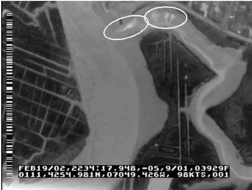
Figure 6: Groundwater Discharge Location TM0005.1.3
