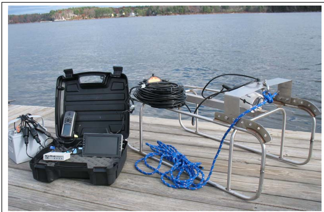
Fig. 2. Towed underwater video system showing major components when deployed in sled mode (see text for details).
