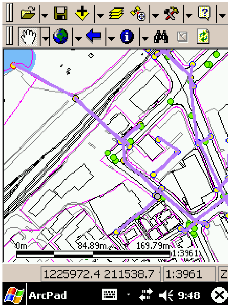
Figure 3: Using a handheld computer, Portsmouth staff sketched the pipes (purple) that connected catchbasins, manholes, and outfalls.
