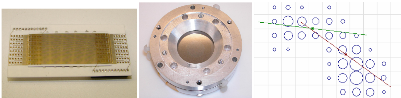
Figure 2.1 Left: Readout strips. Centre: The multiplication stage of a micropattern proportional counter. Right: A reconstructed track from a 6 keV X-ray interaction in Ne:DME. The red line shows the emission angle derived from a one-stage algorithm using the entire track. The green-upper line represents the angle derived from a two-stage algorithm and is significantly more accurate; the grid is on a 132 \mu\text{m} spacing.
