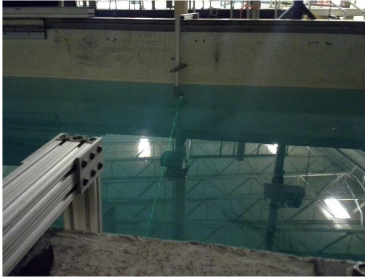
PHOTO 1: UNH OCEAN WAVE AND TOW TANK. 1 DIMENSIONAL TEST OF DETECTOR UNIT AND TRANSMITTER UNIT IN WATER.
