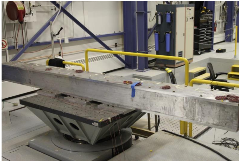
Figure 3: Sandia National Laboratory shaker with expander and basket (McConnell et al., 2013)
