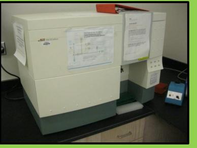
Flow Cytometry: Each solution sample is run through a flow cytometer. This machine uses laser scattering to detect the size, granularity, and fluorescence of individual cells. These properties are directly proportional to the amount of light that is scattered.
