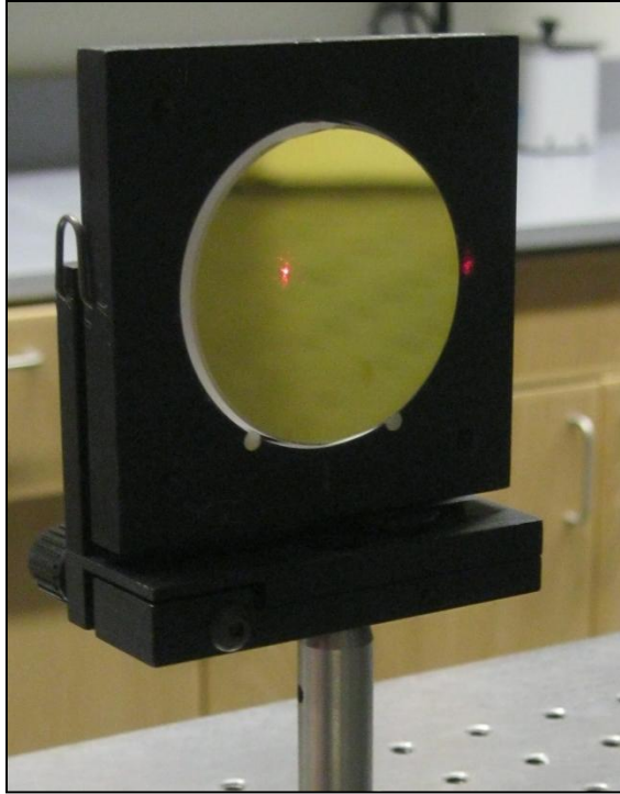
Figure 10a: The Back Reflector. Here, a small spherical mirror is mounted on an angular stage. Using two knobs on the back of the stage allows control of the angle in two directions, with accuracies of about 10^{-3} radians. Also note the red laser dot from the laser pointer, which is the light that has gone through the spatial filter and is now reflecting off. Technically, there should be no side reflections, but the spherical mirror available had a lot of scratches on its surface, which cause losses in the system. The flat mirror is also on a similar angular stage.
