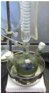
Figure 4.3: Experimental Setup for the extraction of microalgal lipids using either hexane or heptane.
