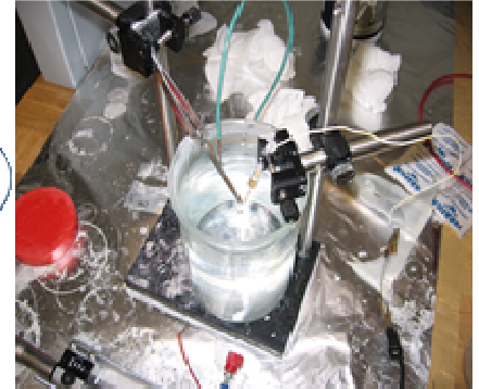
Fig.2: On the right is a photo of the apparatus used to sharpen tungsten wire. On the left is a diagram showing its structure and different parts.
