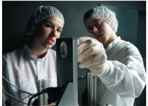
The authors calibrating the star sensor in UNH’s Facility for Optical Calibration at Low Light Levels in 2007 (David Sims, UNH-EOS.)
