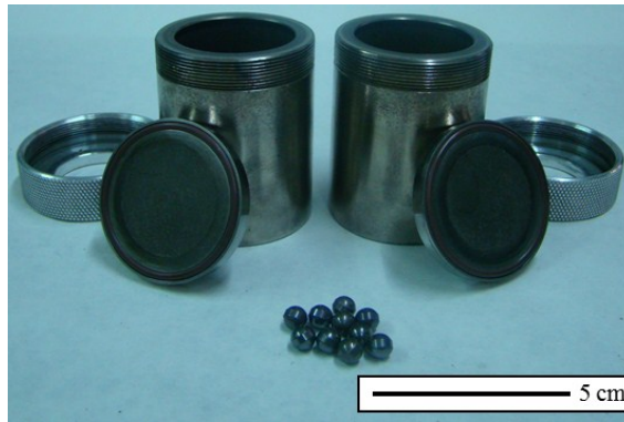
Figure I.3. Milling containers and WC balls used for the high-energy ball-milling of the powders.
