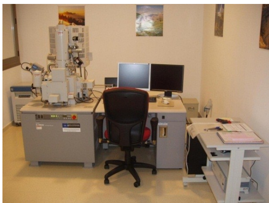
Figure I.7. Field-emission gun scanning electron microscope with an energy dispersive X-ray spectrometer used for the microstructural characterization.
