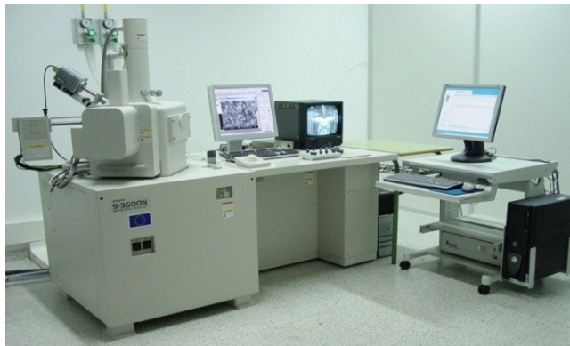
Figure I.6. Conventional scanning electron microscope with an energy dispersive X-ray spectrometer used for the microstructural characterization.
