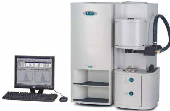
Figure I.9. Inert gas fusion equipment used to determine the oxygen contents in selected powders.
