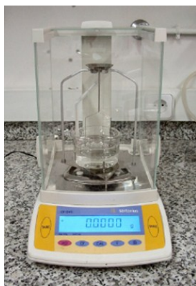
Figure I.14. Analytical balance with hydrostatic weighing equipment used to measure densities by Archimedes' method.
