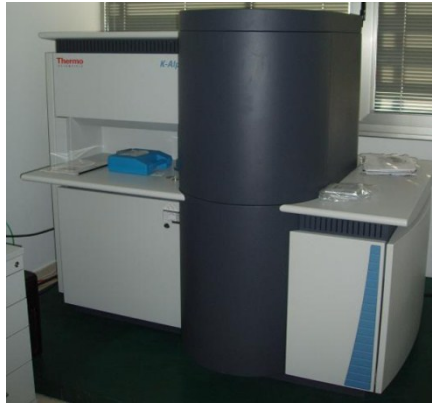
Figure I.13. X-ray photoelectron spectrometer used for the determination of chemical status in selected powders.
