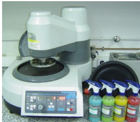
Figure I.18. Polishing machine, synthetic woven clothes, and diamond suspensions.
