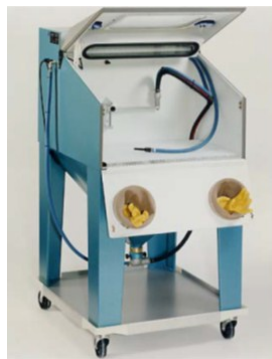
Figure I.17. Surface shoot-peening machine used to clean the sintered samples.
