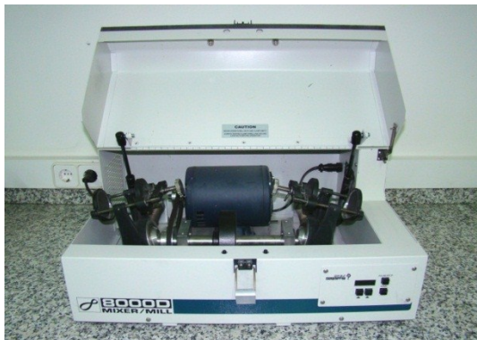
Figure I.2. High-energy shaker mill used for the powder milling.
