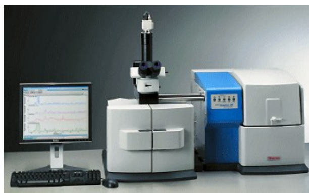
Figure I.12. Micro-Raman spectrometer used for the determination of the bonding environment in selected powders.
