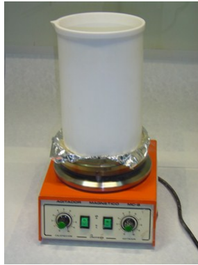
Figure I.1. Beaker and hot-plate used for the homogenization of the as-received powder mixtures and drying of the ceramic slurries.
