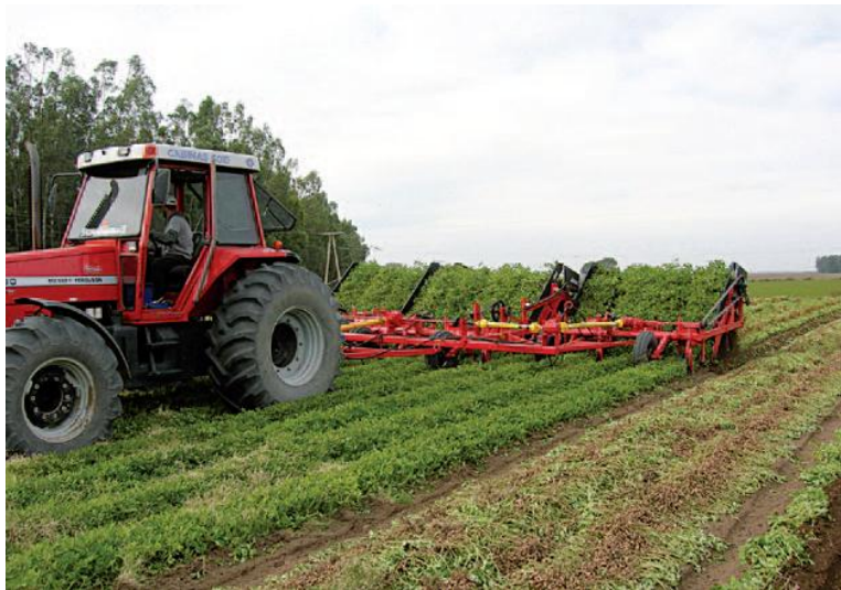
Figura 4.2 Arrancadora invertidora (tomado de http://www.ciacabrera.com.ar/docs/Mani,%20Guia%20practica%20para%20su%20Cultivo.pdf )
